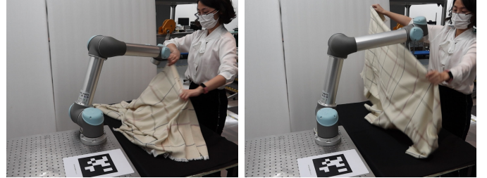
Fig. 1: The real-world assembly task. Left: a robot controller without human awareness, and the robot interrupts human’s work. Right: our human-aware robot controller and the robot leaves human workspace clear while moving towards the target.
