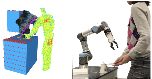
Fig. 1: Close proximity human-robot collaboration by sharing a simulated environment (left) and a real-world scenario (right).
